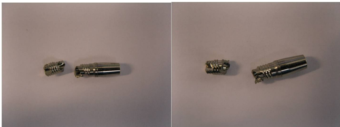
Figure 28. Fractured Implant from Fatigue Test with Maximum Load of 700 N Failed at 3,600 Cycle (Left) and Failed at 3,600 Cycle (Right)
